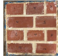
Brickwork specimen with an English bond pattern
