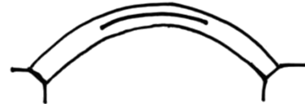
Ring separation under cyclic loading
