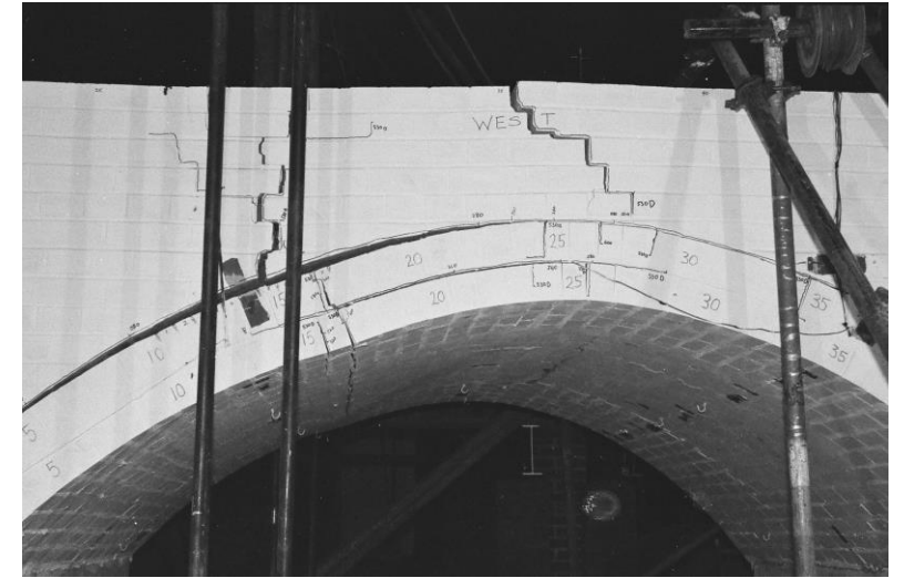
Experimental Crack Pattern (Melbourne & Gilbert, 1995)
